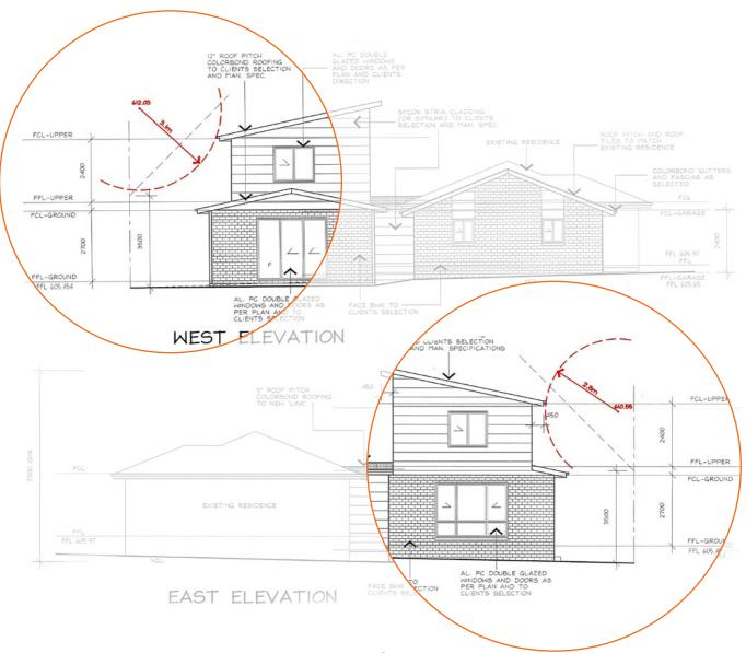
If clearance to existing conductors cannot be met in accordance with Evoenergy drawing requirement 3811-004 to the low voltage network, it may be possible to convert these open wire conductors to insulated bundled conductors at the developer's expense. For more information on this contact network.connectionadvice@evoenergy.com.au
