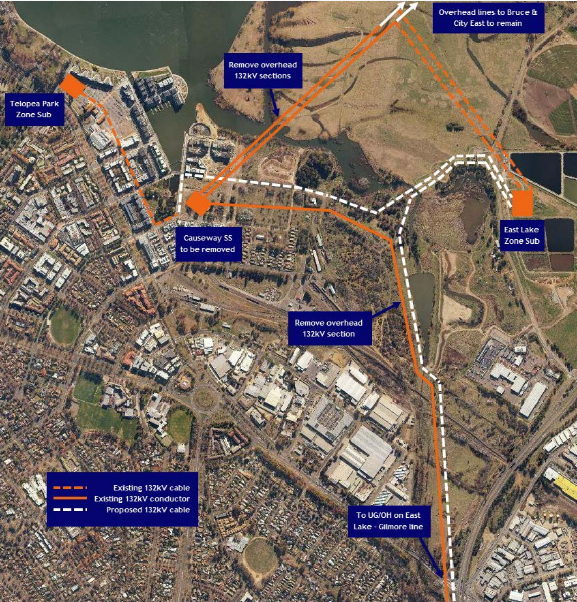
Figure 37. Causeway Switching Station – Proposed 132kV Cabling
