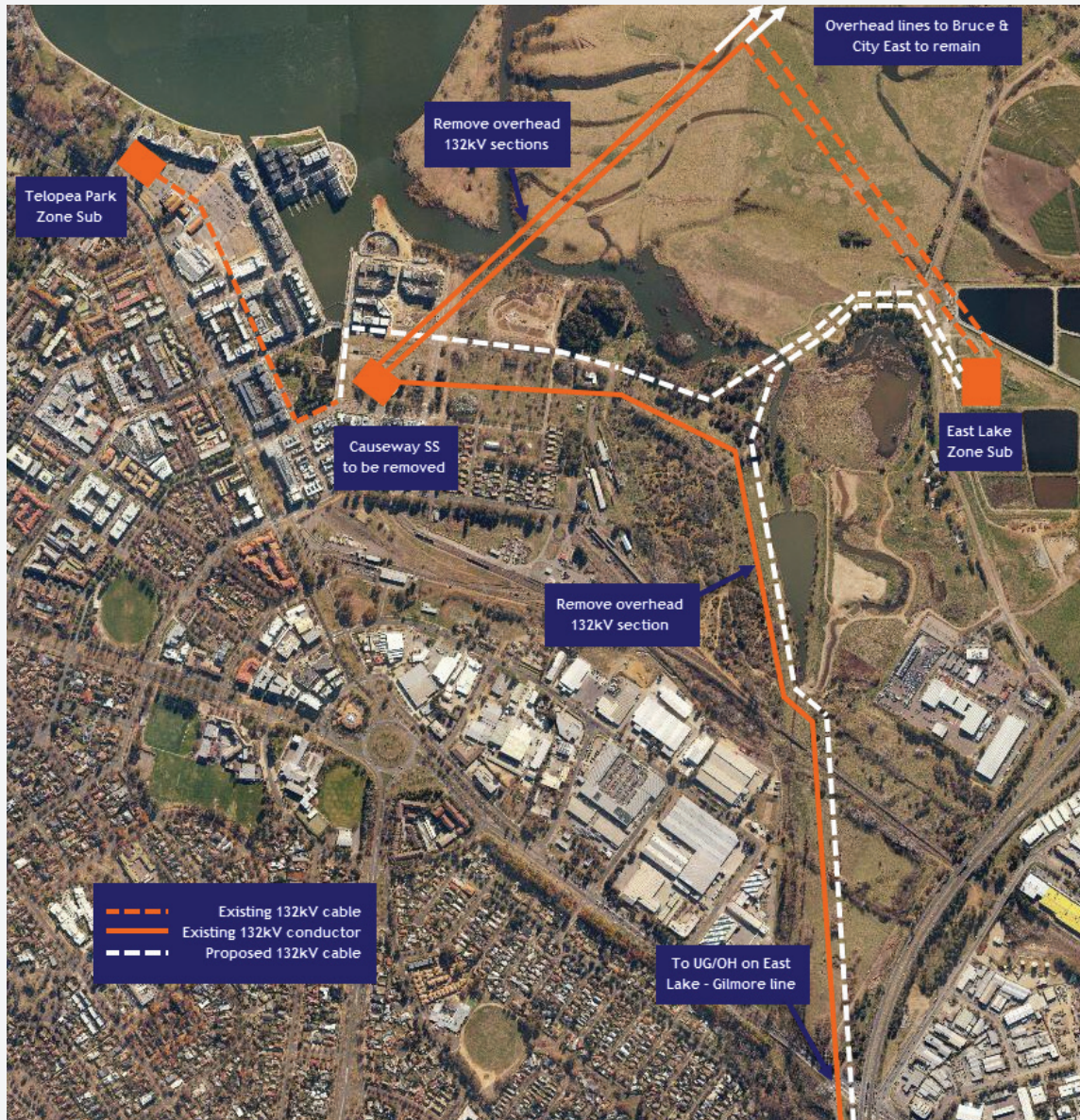
Figure 33. Causeway Switching Station – Proposed 132 kV Cabling
